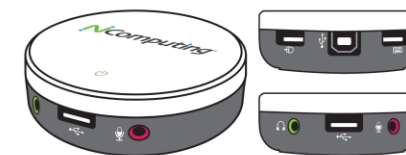
Optional XD4 dongles to expand available USB ports
